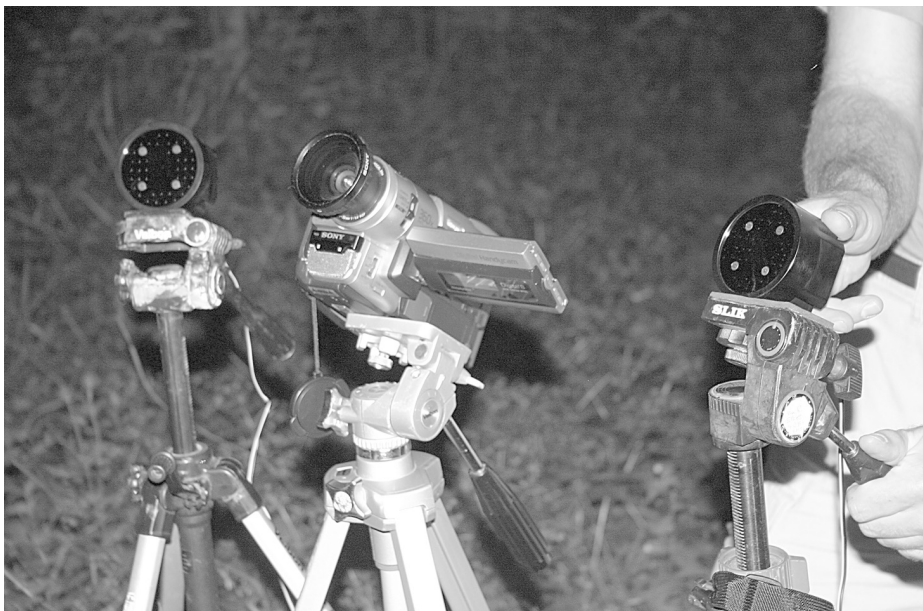
Figure 1. Video set up with Sony Digital8 video camera and Wildlife Engineering NIR lamps.
