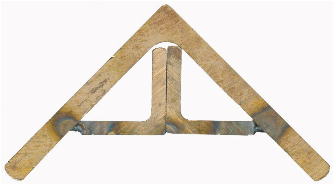
Cross-section of 4-inch angle-iron bar with 1½-inch stiffeners welded inside (to scale).
