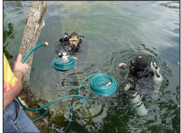
Figure 3.(a) Cave divers handling two lengths of the sample tubing at the cenote surface.
