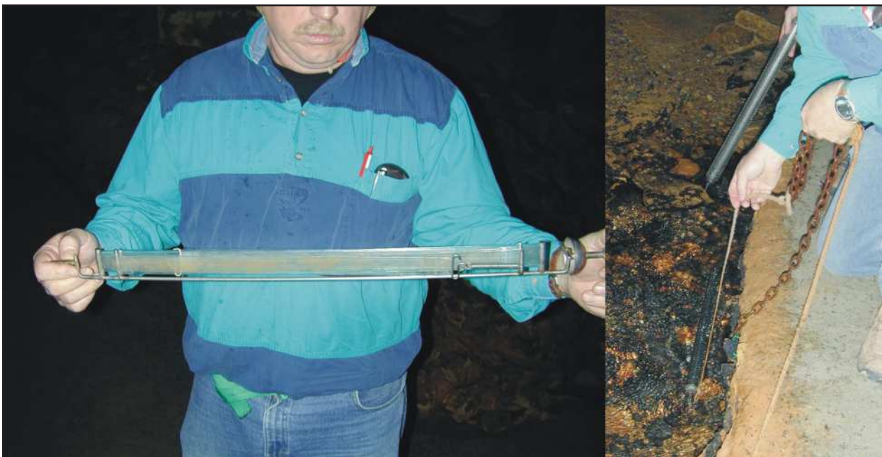
Figure 4 SPMD deployed by William R. Elliott in Tumbling Creek Cave. The membrane sampler is inserted into a perforated cover and anchored in the stream. Photo by Steve Samoray.
