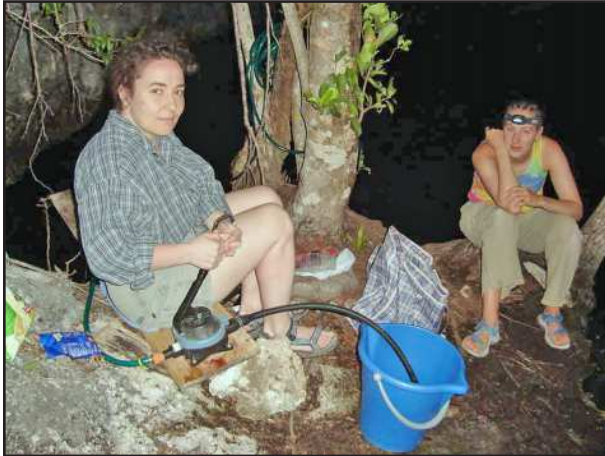
Figure 3(c) Manual pumping of water samples from a fixed point in the water-filled cave. The internal volume of the tubing is voided into the bucket before each sample.
