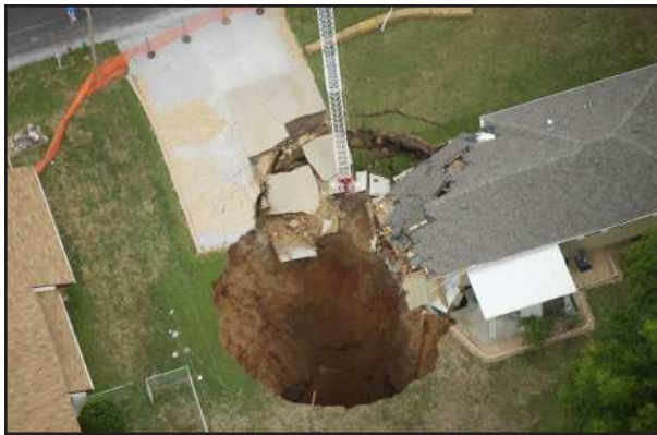
Figure 11 Aerial view of the a collapse at 327 N. Delaware Avenue, Nixa, Christian County, Missouri, beneath part of a house owned by Mr. Norman Scrivener. The depth of the structure was measured at about 25 m (75 ft.). This was after engulfing the garage, which included a medium-sized sedan.
