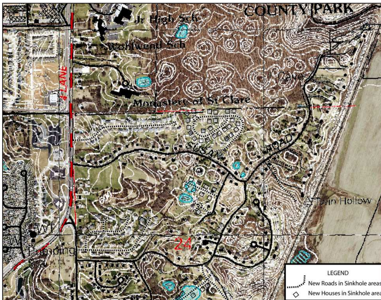
Figure 5 Topographic contours (white, from Oakville 7.5" map 1991) superimposed on a recent satellite image (USGS Urban Area Imagery, March 2004) of an area within and immediately south of Cliff Cave County Park. Many houses and roads have been constructed on filled sinkholes and sinkhole ponds, and others are directly above caves.
