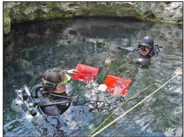
Figure 3(b) Pre-dive briefing on the dye-release protocol showing the two heat-sealed, impermeable cloth pouches containing masses of dye. These are cut open with utility shears underwater.
