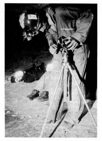
Figure 3. A Brunton compass is used to determine the vertical angle and azimuth of the camera face.
