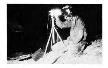
Figure 2. The camera and tripod are centered over the photo point marker using the plumb bob.
